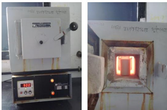
Fig.4 Low temperature heating at 900°C
