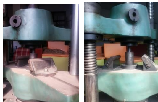
Fig.2 Pellet casting using compaction method
