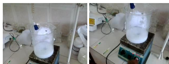
Fig.1 Zirconia powder preparation using simple co precipitation method.
